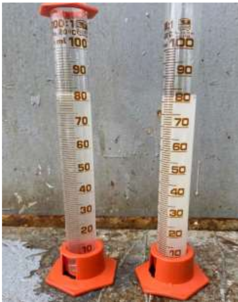
Figure 9: FET test after 8 hours, without dispersant (left) and with dispersant (right).
